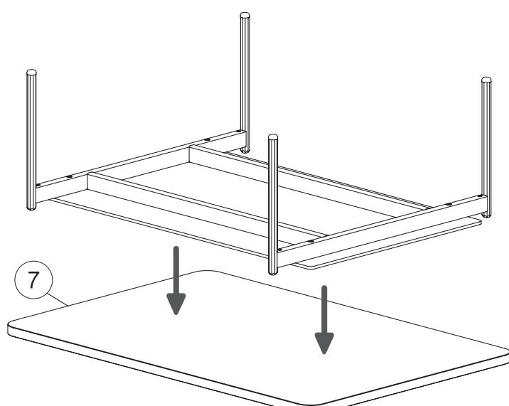
**EN** - Place the marble top (7) on a smooth and anti-scratch surface, turn the coffee table upside down centering the marble top to the panel. Let the adhesive sealant dry for 48 hours without moving or touching the coffee table. After 48 hours turn the table upside down without forcing the top.
