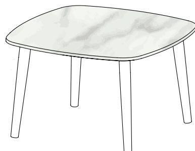
**EN - ! WARNING!!!** Pedrali refuses any responsibility for tops not assembled according the directions; or rather screws without using silicone or used without waiting 48 hours after its application. The use of automatic screw drivers is unadvisable.
